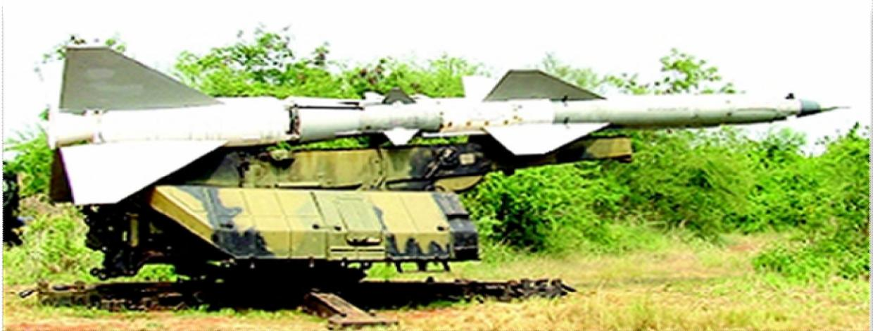
**SM-90 Rocket Launch Pad.** It is part of the **Volga Anti-Aircraft Rocket Complex**. It is used for the preparation before the launch of rockets **20DC** and **5A23**. It reaches 15 000 m.
