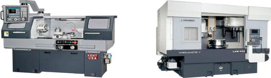
Torno CNC Horizontal | Torno CNC Vertical
